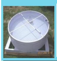
**Pan Material** Copper / GI / SS **Pan Diameter** 1220 mm ±3 mm User select the pan material and standard before Getting Quotation
